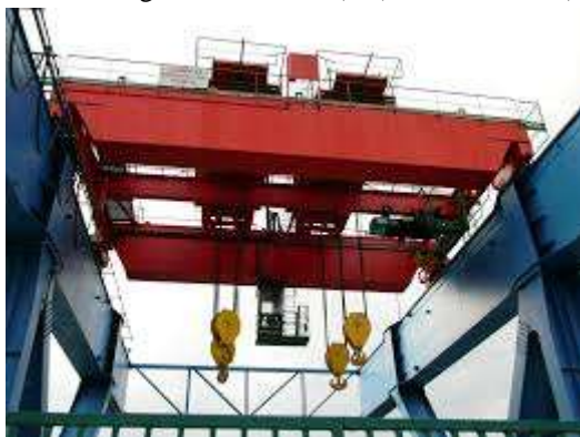
Fig 1: Overhead travelling crane
